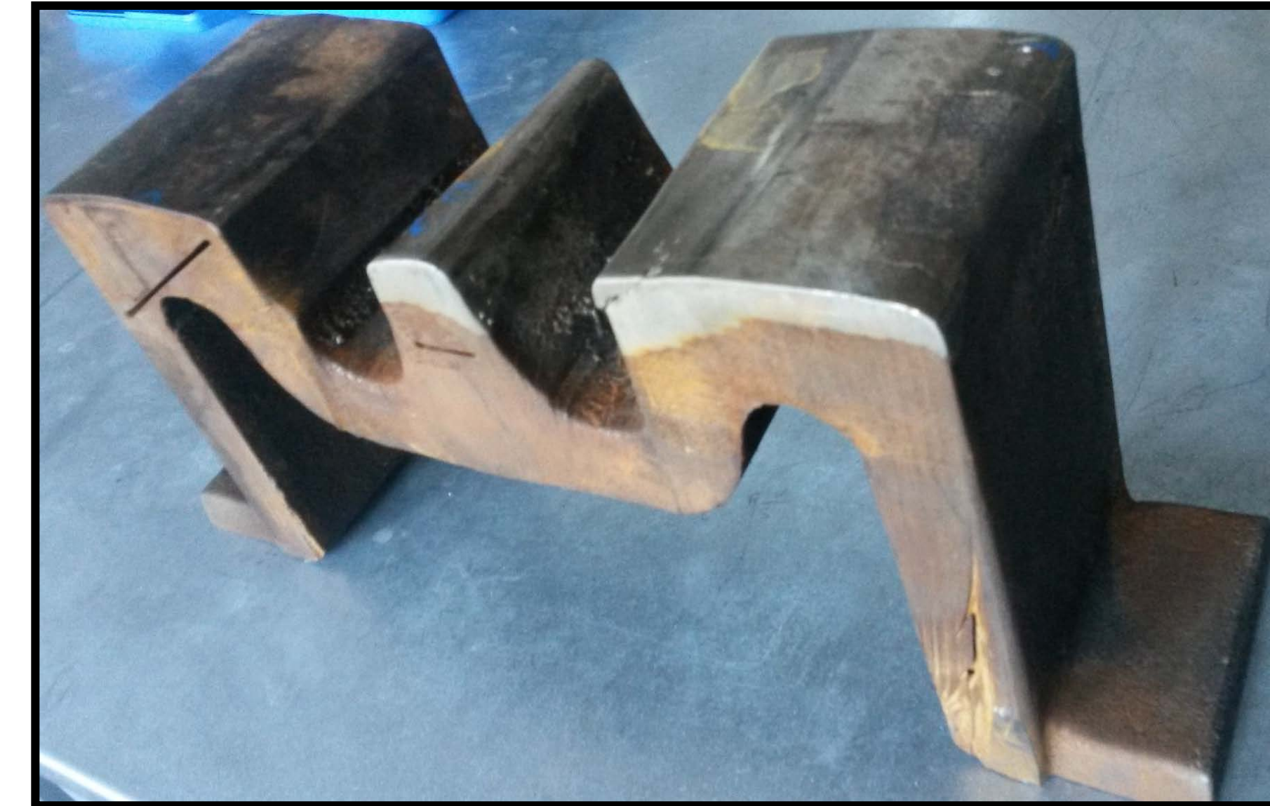
Section of a railway crossing.
