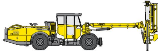
Figure 8. Simba, Long hole drill rig (Courtesy Epiroc)
